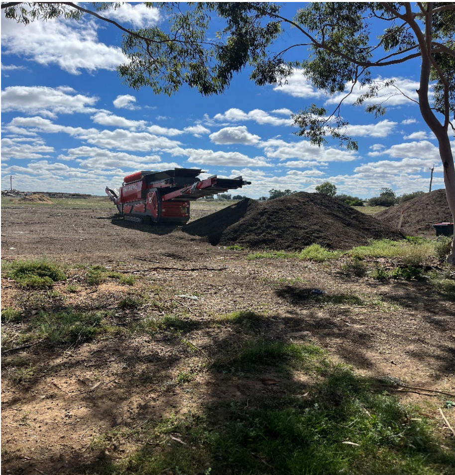
Trommel for grading the soil enhancer
